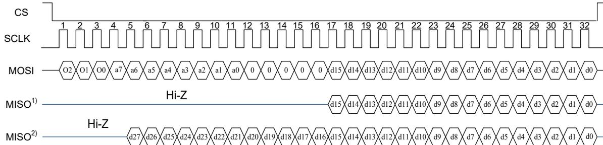
Figure 4. SPI data output sequence diagram
