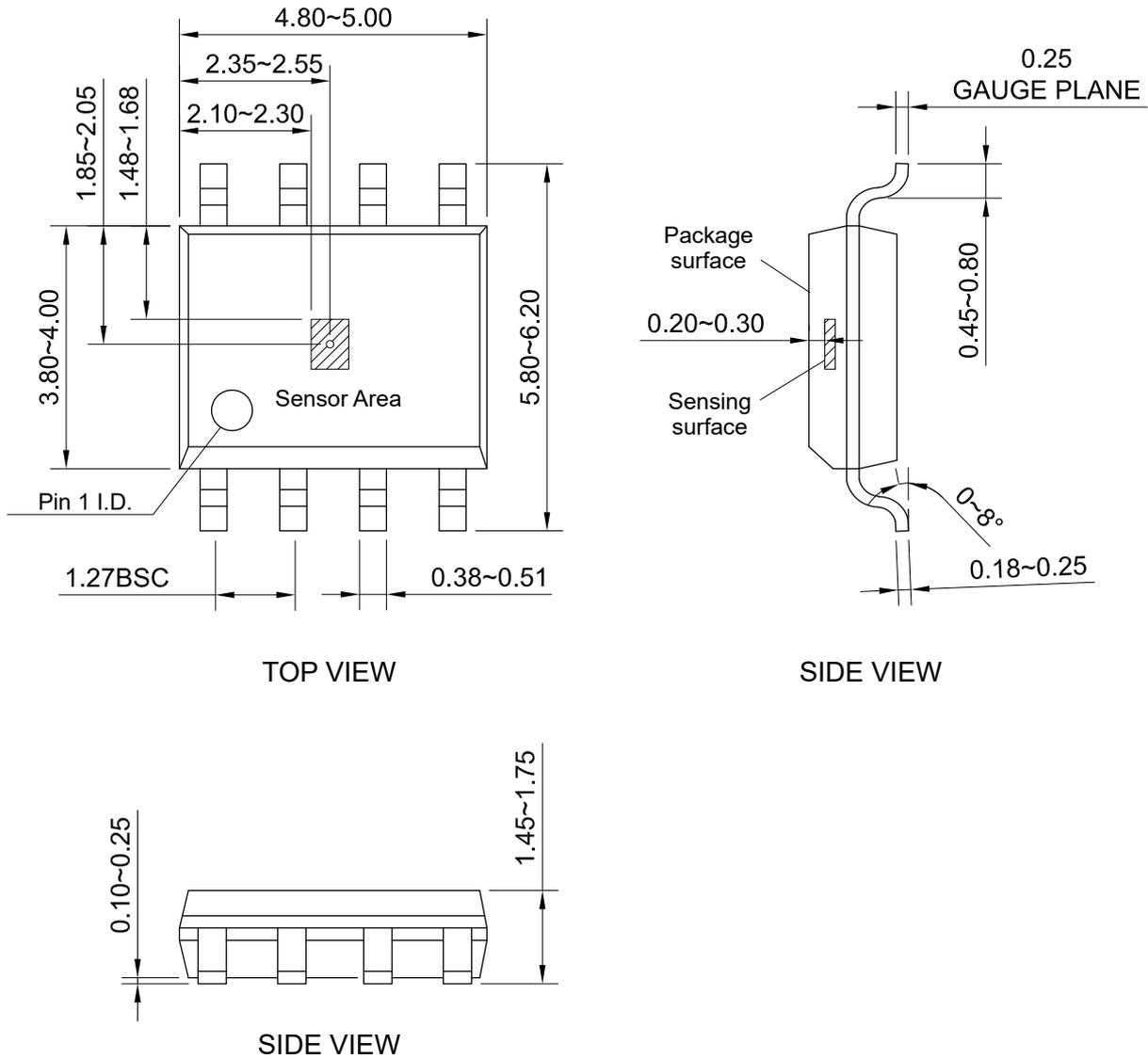
Figure 17. Package outline of SOP8 (unit: mm)
