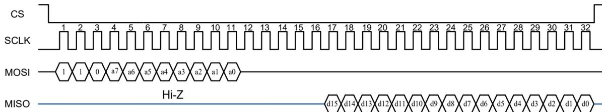
Figure 7. SPI write register sequence diagram
