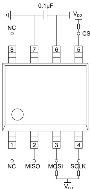
Figure 14. Schematic of 4-wire SPI circuit
