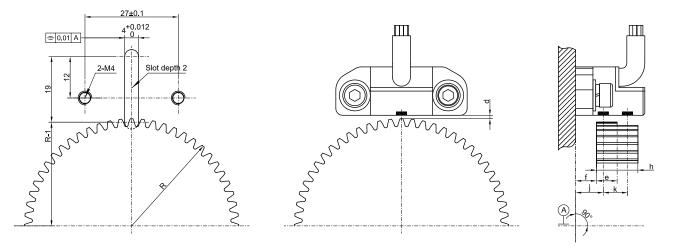
Figure 8. Mounting schematics (unit: mm)
