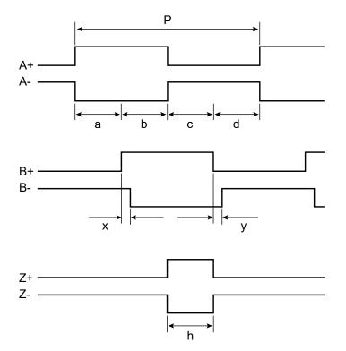
Figure 1. TTL differential square wave signals
