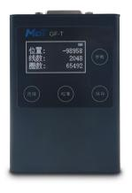
Figure 4. Diagnostic tool GF-T for GE-T encoder only
