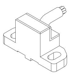
Figure 7. Outline of GE series encoder (unit: mm)
