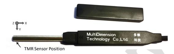
The USB magnetometer hardware is compatible with the popular open source Arduino UNO board, and thus with the Arduino programming environment or Atmel microcontroller development tools. The user may develop custom firmware at his/her own risk. The hardware includes a boot loader for uploading Arduino code. The USB magnetometer hardware model is defined as follows:
