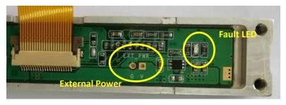
Figure 1. External Power Connection
