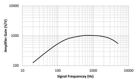
Figure 2. Band-pass amplifier transfer characteristics
