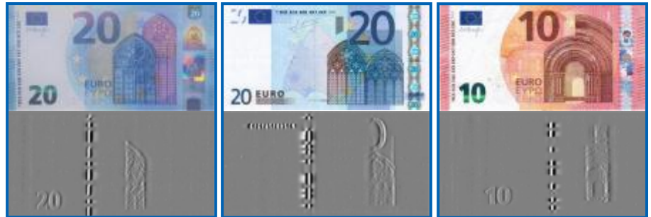
Magnetic Image of MDT's 50DPI Magnetic Image Sensor
